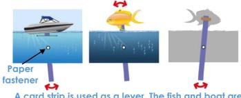
A card strip is used as a lever. The fish and boat are glued to the lever which is used as a handle.
